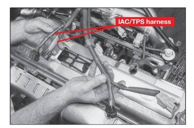
b. Carefully cut open the main wire harness wire loom to provide enough harness slack so the TPS and IAC connectors can reach the relocated throttle body.
