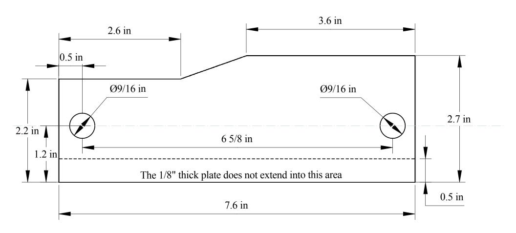
This plate is made up from a 3/16" plate and a 1/8" backing plate (1/2" narrower - refer dotted line) The 1/2" narrower backing plate is to clear weld area of one of the toyota body mount outriggers
