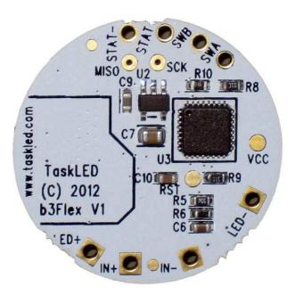
The picture shows the connections to b3Flex V1.0. The user provides DC power to the b3Flex (via battery or DC adapter). b3Flex is reverse polarity protected with a low drop out FET (less than 50mV voltage drop across the FET).
