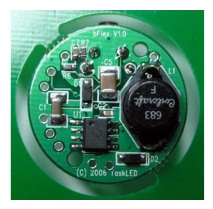
As shipped, the bFlex is configured for nominal 350mA drive. The user may reconfigure the bFlex drive level as described later in this document.
