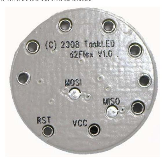
When soldering wires to the through holes/pads on the PCB, be careful to not short or accidentally desolder components near where you are soldering. Use a quality solder with non-corrosive, non-conductive (no clean) flux. Do NOT try to drill out or expand the holes.
