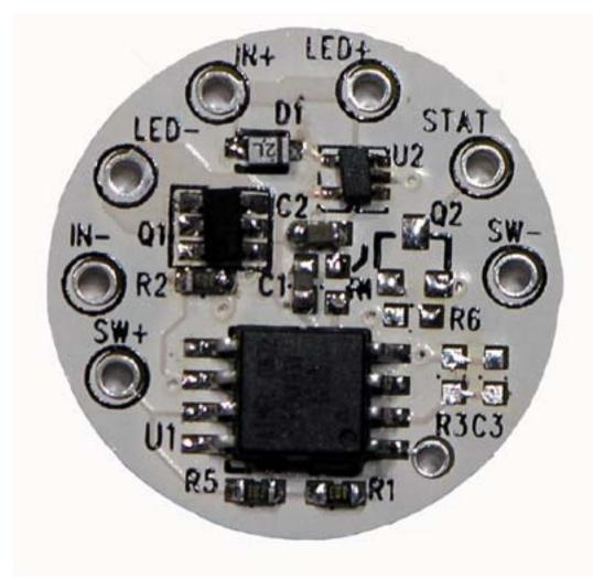
The picture shows the connections to d2Flex. The user provides DC power to the d2Flex (via battery, DC wallwart, vehicle/boat/RV 12V. d2Flex is reverse polarity.
