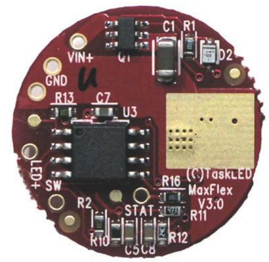
The picture shows the connections to maxFlex3. The user provides DC power to the maxFlex3 (via battery, DC wallwart etc.
