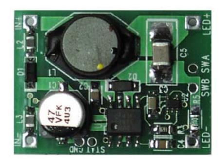
The picture shows the connections to the nFlex. The user needs to provide DC power to the nFlex (e.g. battery, DC wallwart, vehicle/boat/RV 12V).
