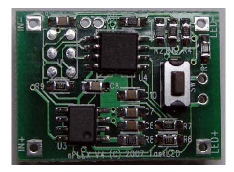
The picture shows the connections to nFlex. The user provides DC power to the nFlex (via battery, DC wallwart, vehicle/boat/RV 12 V). nFlex is reverse polarity protected.
